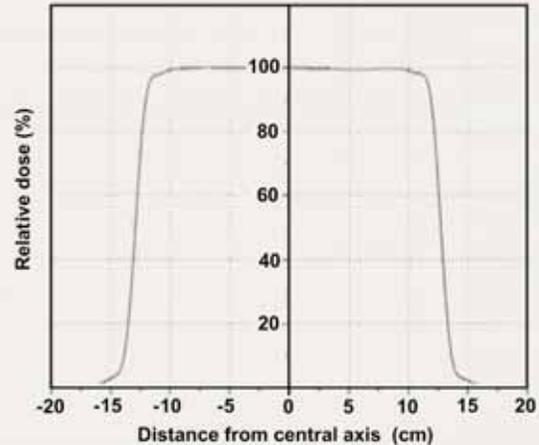
*Dose profile measured at a depth of dose maximum  $z_{max}$  in water for a 12 MeV electron beam and 25x25 cm<sup>2</sup> applicator cone.*
